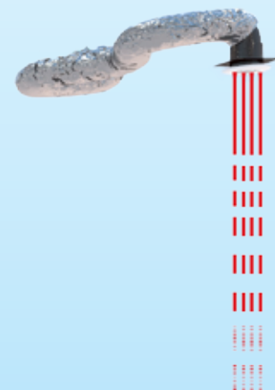
Air is delivered in a concentrated column causing the room air to mix evenly.
